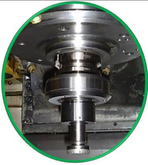
Vertical machining center manufactured by O company Automatic balancer “zero core” tool Electroplated grindstone installation diagram
